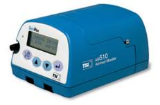
real-time concentration of particles smaller than  $2.5\mu m$  in micrograms per cubic meter, or PM<sub>2.5</sub>. The SidePak was calibrated against a light scattering instrument, which had been previously calibrated and used in similar studies. In addition, the SidePak was zero-calibrated prior to each use by attaching a HEPA filter according to the manufacturer's specifications.
