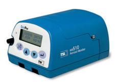
real-time concentration of particles smaller than  $2.5\mu m$  in micrograms per cubic meter, or  $PM_{2.5}$ . The SidePak was calibrated against a light scattering instrument, which had been previously calibrated and used in similar studies. In addition, the SidePak was zero-calibrated prior to each use by attaching a HEPA filter according to the manufacturer's specifications.
