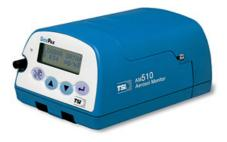
the device and the particulate matter in the air scatters the light from a laser to assess the realtime concentration of particles smaller than  $2.5\mu m$  in micrograms per cubic meter, or PM<sub>2.5</sub>. The SidePak was calibrated against a light scattering instrument, which had been previously calibrated and used in similar studies. In addition, the SidePak was zero-calibrated prior to each use by attaching a HEPA filter according to the manufacturer's specifications.
