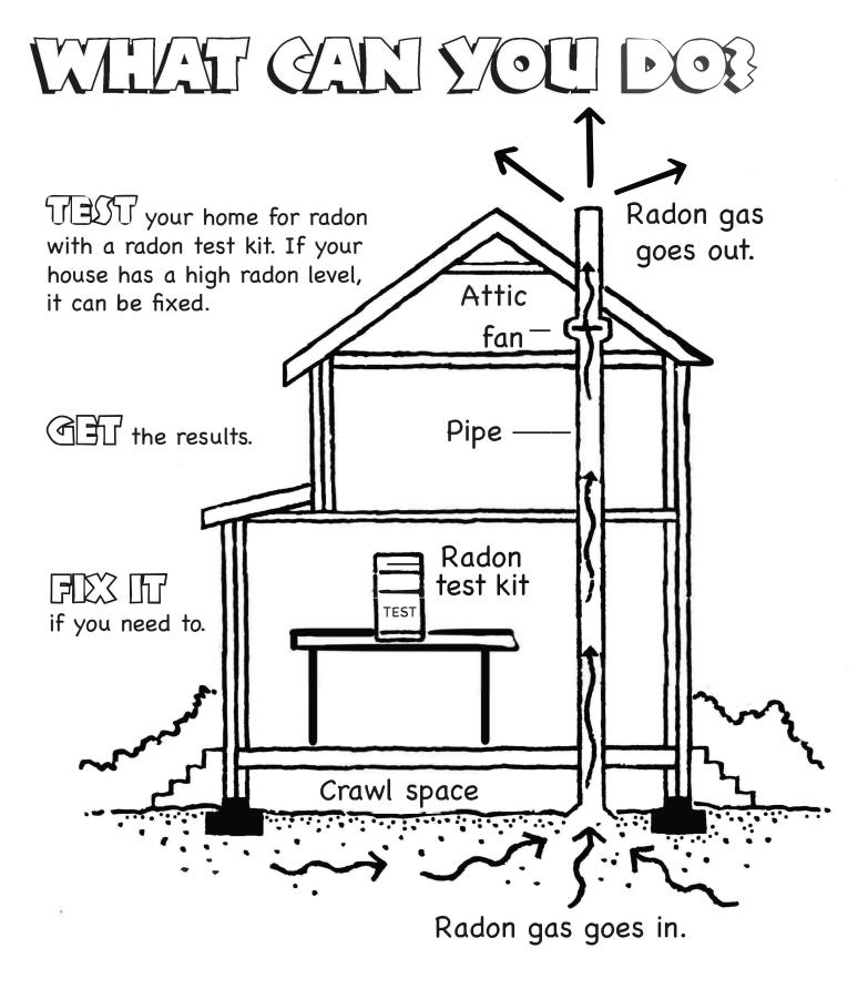
A **MITIGATION SYSTEM** is a pipe and fan that helps remove radon gas from your home.
