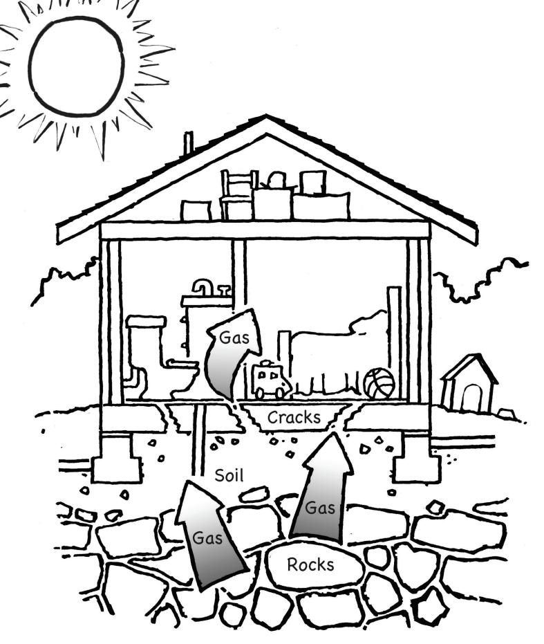
Sometimes radon gas enters a house from **CRACKS** in the foundation and openings around pipes.
